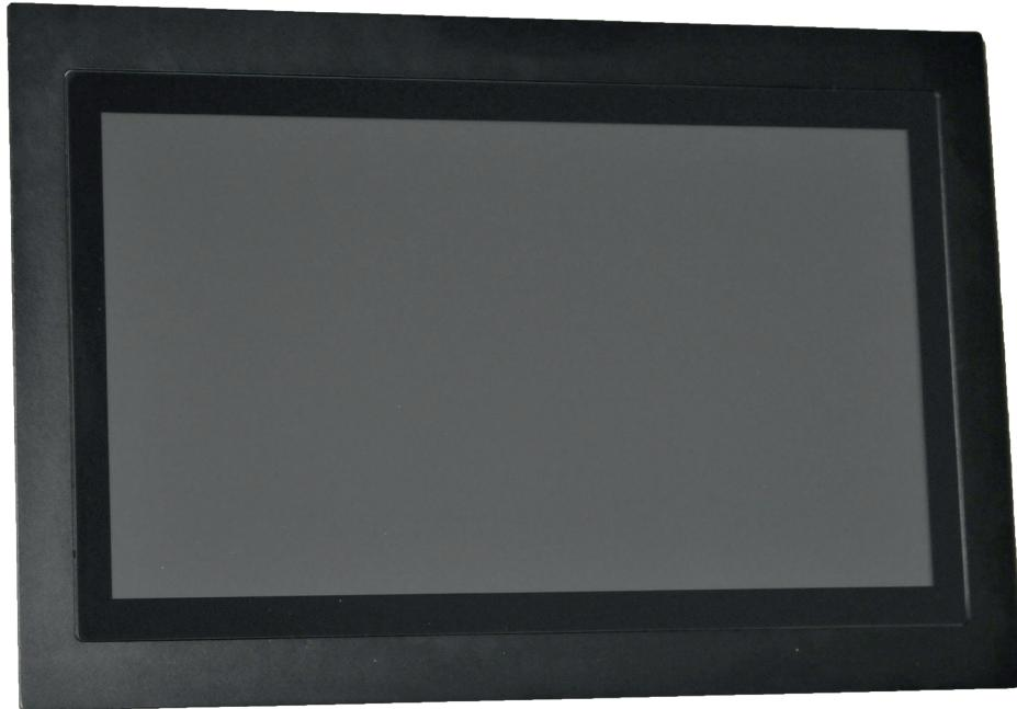
**21.5“ TFT LCD Monitor with PCAP Touch and metal frame.
